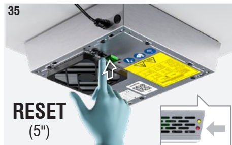
Fig. 39: Keep the reset button pressed for at least 5 seconds until the alarm led (red led) goes out.
