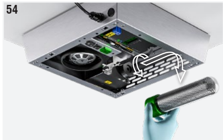
Fig. 54: Gently unscrew the ionizing tube by grasping it at the base (green part).
