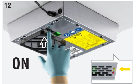
Fig. 12: Set the switch to ON to check for voltage in the device. If the installation is correct, the yellow LED lights up and the red alarm signalling LED does not light up.
